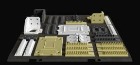
Element HT can print high-strength parts with tight tolerences.
